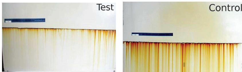
Fig. 4: Visual inspection of the galvanized steel test panel and control panel
