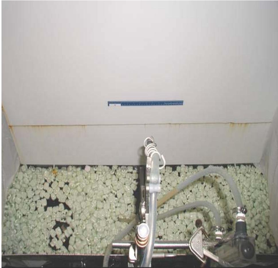
Figure 4: View of test system from above the nozzle stand. The scribe in the panel is shown as the rust line across the width of the panel.
